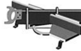
Trim at 45 degree angle. The resulting cut exposes the profile of the moulding, serving as a template. Following this profile with the coping saw at a 90 degree angle to the face of the moulding results in a duplication of the pattern, which fits over the face of the adjoining moulding.
