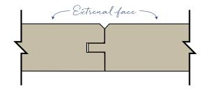
the boards can be fixed mid stud or cavity batten, eliminating the need to dock and create volumes of waste, saving up to 10% of the product that previously would have been thrown away. Not only does this save costs, it's a better for our environment with less resource being used.
