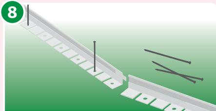
8 Check that the position of the Link Edge is visually correct. If it is not, remove the spikes and reposition it
