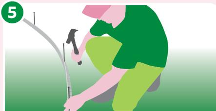
5 Half hammer subsequent spikes in pivotal areas along the length (especially at points where a bend or curve is required).
