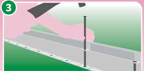
If using 75mm, 100mm or higher Link Edge, use spike guides to provide extra upright rigidity. Ensure edge spike hole is towards the bottom of the spike guide.
