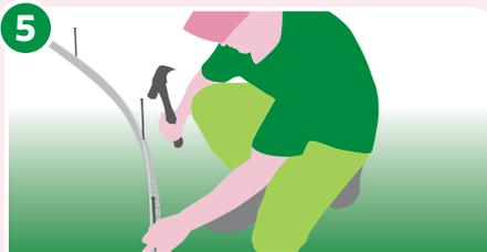
Half hammer subsequent spikes in pivotal areas along the length (especially at points where a bend or curve is required).
