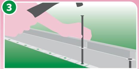
3 If using 75mm, 100mm or higher Link Edge, use spike guides to provide extra upright rigidity. Ensure edge spike hole is towards the bottom of the spike guide.
