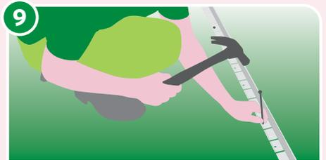
Once satisfied with the positioning of the Link Edge, hammer the spikes firmly into the ground.
