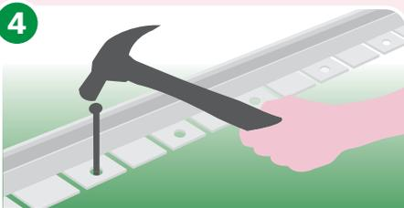
4 Half hammer spikes into pre-punched holes (approximately 1-2 spikes per lineal metre) starting from the first hole in the end of the Link Edge.
