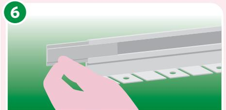
6 Connect any further 3m lengths together by using the fishplate connectors. Slide the fishplate connector into the designated section at the end of the matching length.
